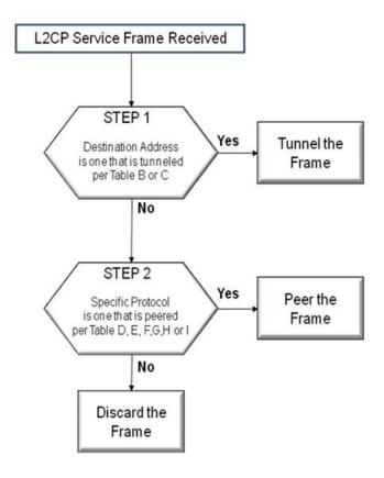
Figure A. The Logic Flow Chart for L2CP Service Frames
